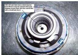
require the long stub axle on one side, otherwise the stub will push in too far and the dust slinger on the stub axle will cut the oil seal. The other problem with some LSD centres, is the fitting of the speedo gear. Some like KAAZ ones require a unique version of the speedo gear to fit their machined casting, while others just don't fit properly and flop about . Even some TRD diffs are terrible in this regard.
