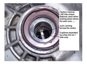
All factory viscous LSD's require special axles with longer splines and different shaft sizes The picture above shows the 2 different LH stub axles, with the long splines on the LSD version being quite obvious. Neither side non-LSD axle can be successfully modified to suit a LSD, but some people have re-ground the RH side and claim it works OK. The factory LSD diff centre has a different speedo gear fitted to it and it won't swap with non-LSD speedo gears.
